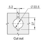
Main material and finish: Bright chromeplated ZDC housing and insert, white zinc-plated steel cam Application: Quarter-turn opening or
